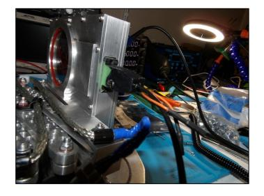
Unplug camera dsub, plug in charging cable to camera case dsub and an external power source and charge the camera for four hours. Replace payload camera dsub when finished. (Step-by-step instructions below; also reference our "Flight Procedures", step 1)
