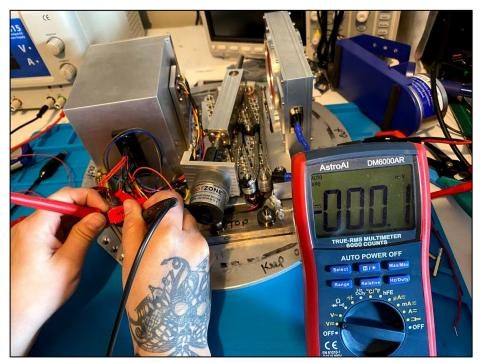
Using multimeter probes and the corresponding power pinout, we verified that there was neutral voltage on all the power pins, including GSE.
