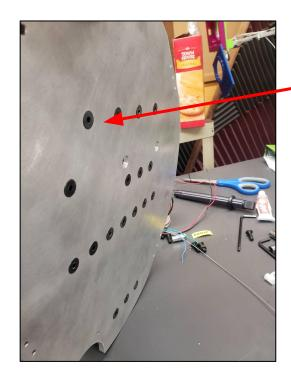
All plate holes countersunk so hardware is flush
