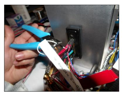
Inhibit (clearly labeled on the Electronics Box d-sub) wire should be cut right before flight. (From our "Flight Procedures", step 3.)
