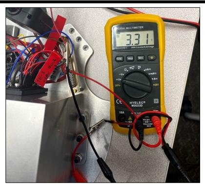
We inserted multimeter probes between our telemetry lines and Ground and ran our code, verifying the voltages of each line.
