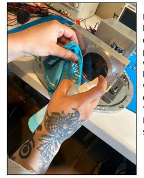
Remove clearly labeled foam camera protector and wipe front and back site glass with cleaner and cloth. (From our "Flight Procedures", step 2)
